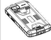
Align the snap joints and press from sides
